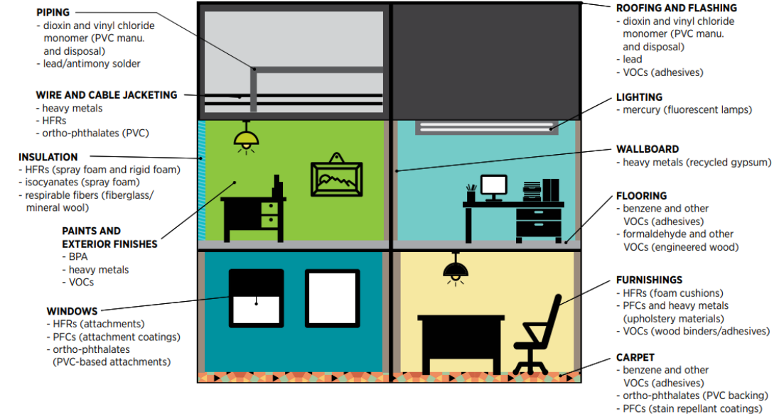
Figure 2-5. Examples of building material ingredients and byproducts that may be harmful during one or multiple stages of the materials life cycle. A typical structure can contain many substances that pose a hazard during the manufacturing phase, use phase, or other stage of the life cycle. Building professionals should be aware of these, and other examples, and evaluate trade-offs between alternative materials.
